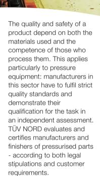
Qualification of manufacturers is described in the Pressure Equipment Directive (PED) 2014/68/EU and applies to pressure equipment and subassemblies subject to pressures greater than 0.5 bar - such as pressure vessels, steam boilers, piping and pressurised fittings with safety functions. TÜV NORD certifies according to the PED and AD 2000-W0, as the national standard of application.
