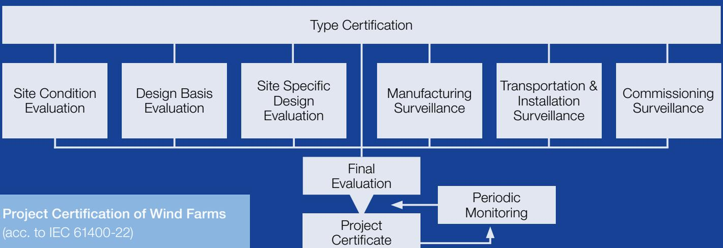
Site conditions such as wind distribution, wind farm effects, temperature, soil and terrain complexity as well as electrical network conditions are evaluated based on applicable measurements and/or local codes.
