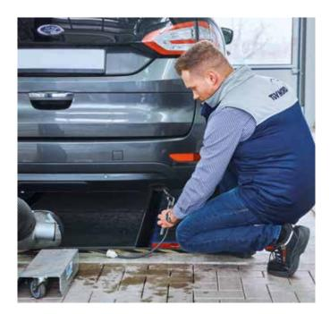
Exhaust gas analysis is an important contribution to environmental protection and to reduce the pollution in our air. That is why the AU is carried out every two years as part of the main inspection. Incidentally, since 2006, the AU has become officially named UMA: Examination of the Engine Management / Emission Control System.
