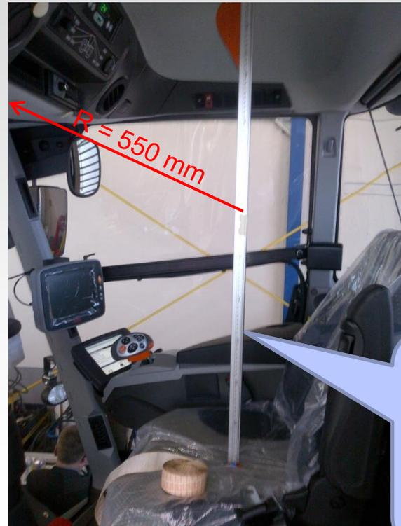
Perpendicular reference axis through centre of ball of the SAB
