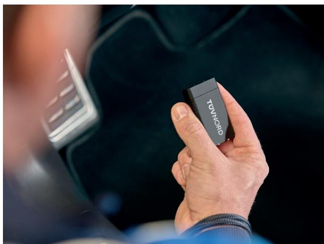
Connect the Guardian to the OBD port in the car (usually found in the driver's footwell on the left side).
