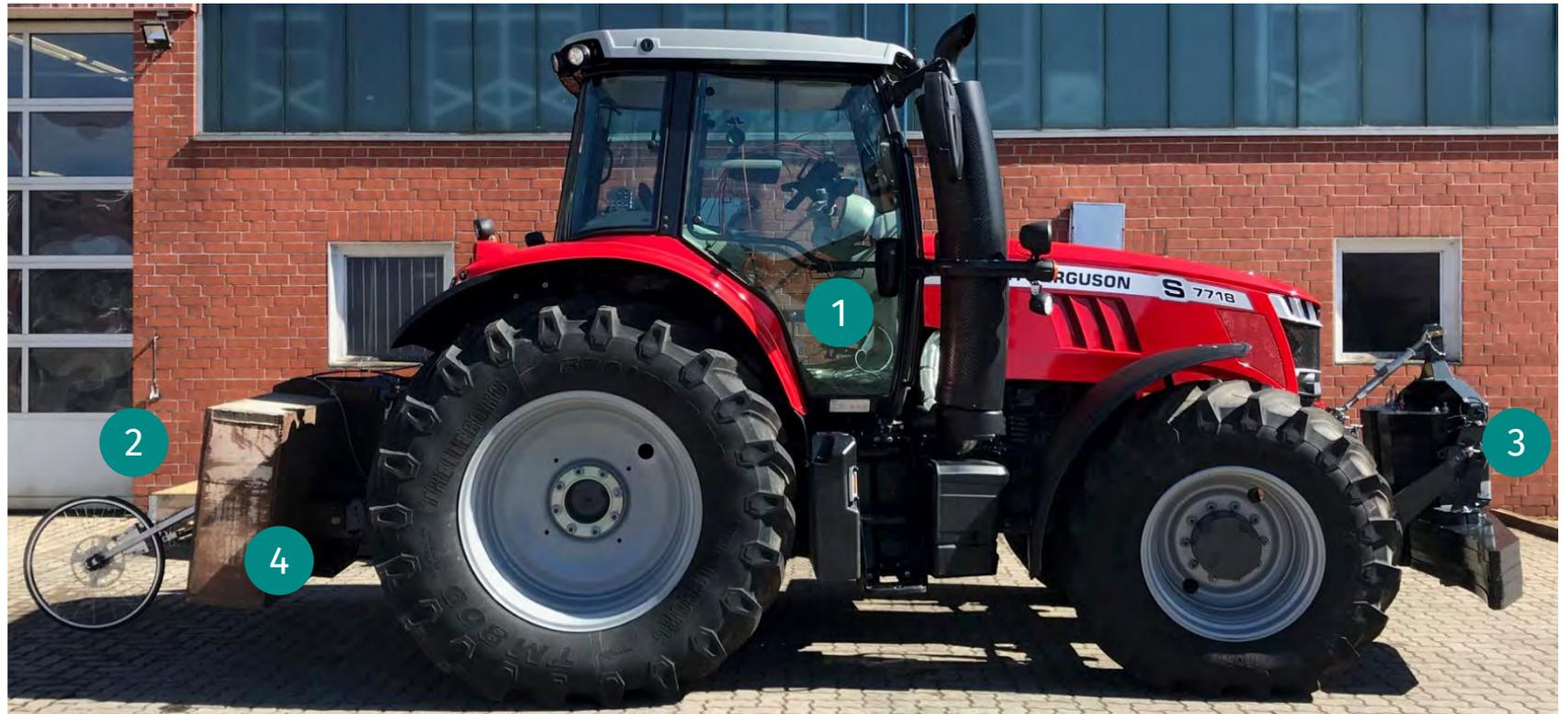
Example of a measurement setup for a loaded tractor
