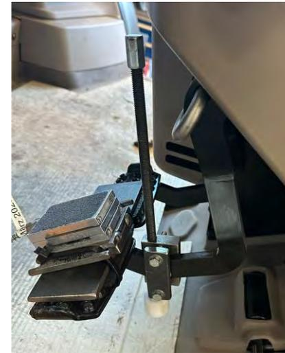
Stopper on brake pedal to receive reproducible measuring results
